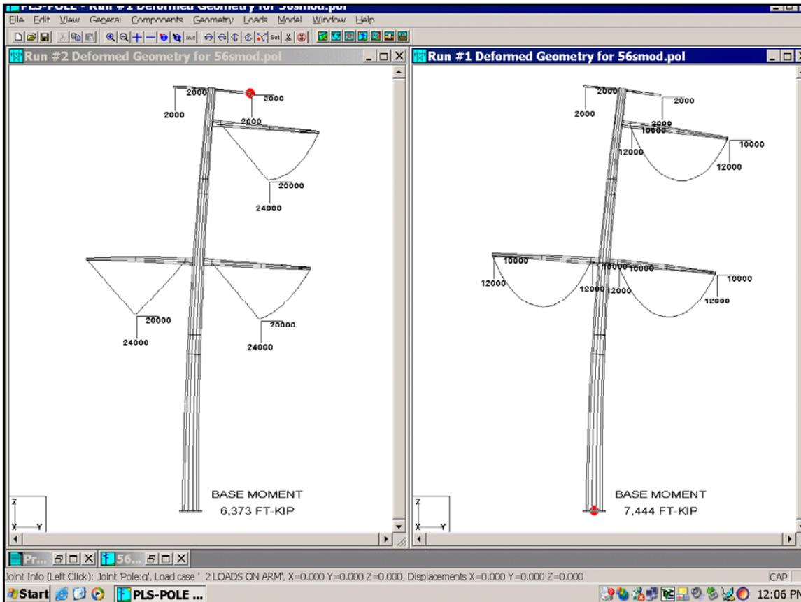
The left pane shows a real tubular pole (displayed at scale) with the load correctly applied to the V-strings and the right pane shows the loads divided equally at the attachment of the V-strings to the arms. A detailed analysis of both models with PLS-POLE shows a substantial difference of 17 % between the base moment in the pole on the left and that on the right.
