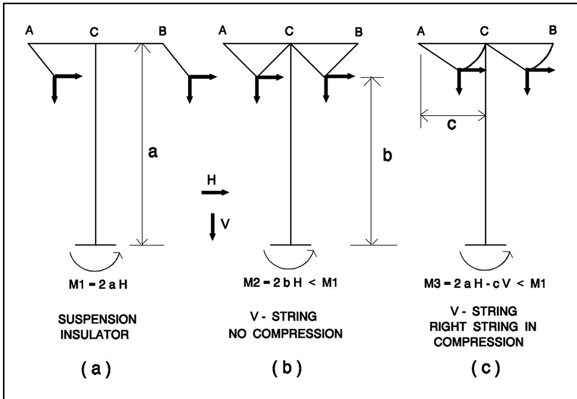
With suspension insulators (left side of figure), the horizontal load H and the vertical load V are transferred to points A and B at the tip of the arms and their effect on the base moment is  $2 a H$ , where a is the height of the arms above the ground.
